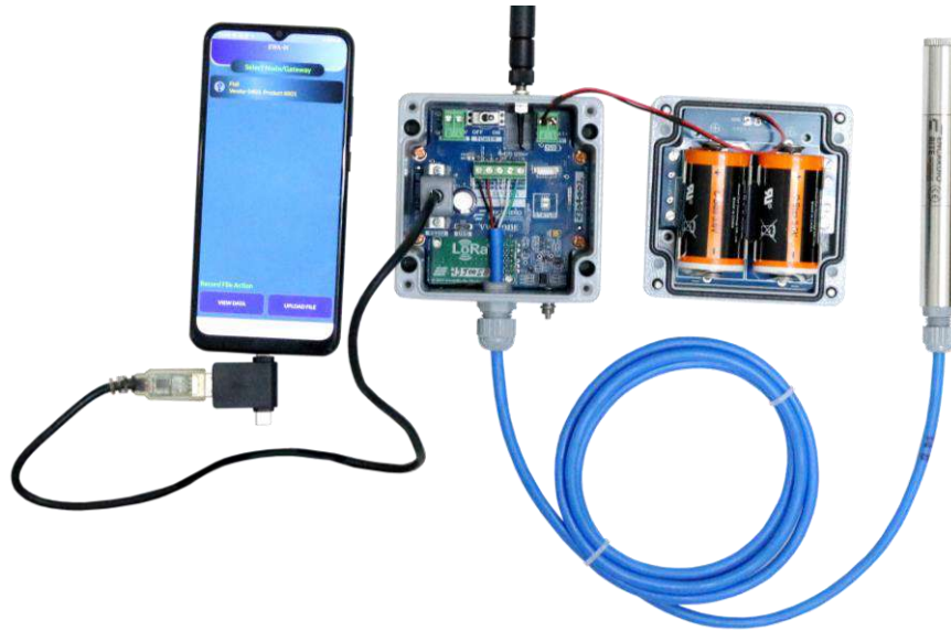
Figure 5-11 EWN-01V VW node connected to Android phone with FTDI cable via OTG adaptor
